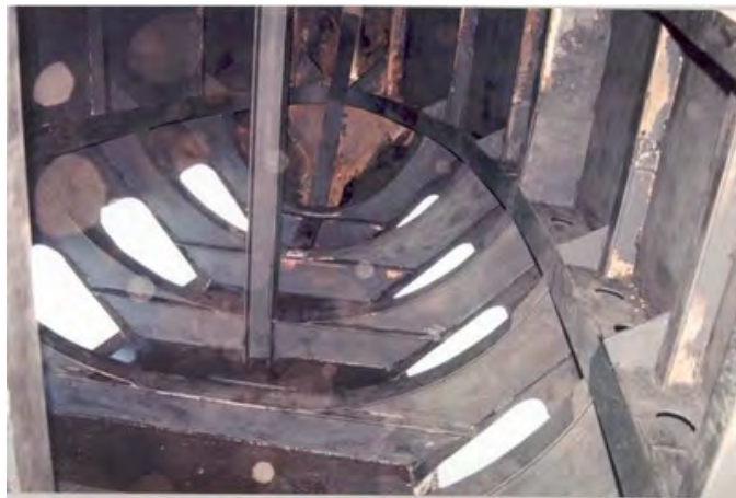
Stem fairing of submarine U.S.S. CROAKER (SSK-246) after completion of structural repairs.
