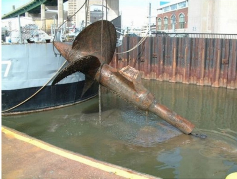
Starboard propeller, portions of the strut and shafting upon removal from destroyer U.S.S. THE SULLIVANS (DD-537).
