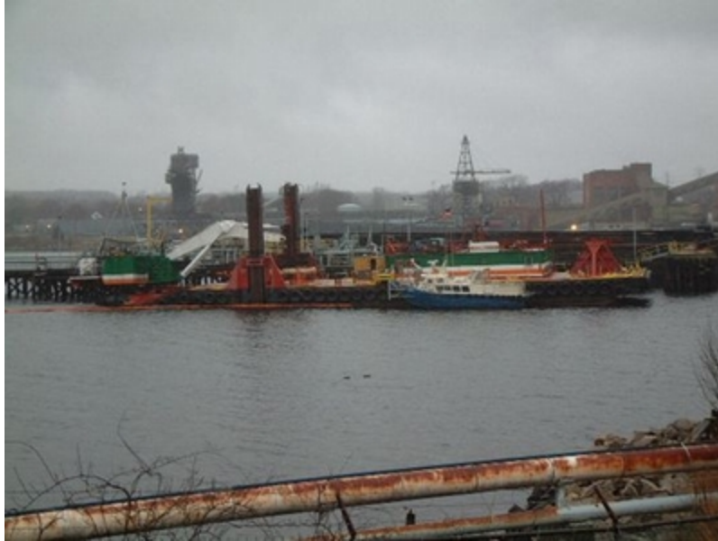
Dredge S. COSMOLETTI, Cashman Equipment Co. mechanical dredge.
